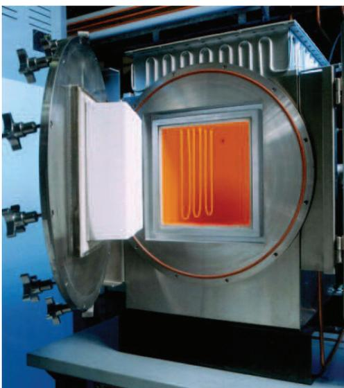
Our client successfully tested a feature of the EPower controller in a new way alongside their world leading brand of (MoSi<sub>2</sub>) heaters known as Kanthal Super. A key feature of MOSi<sub>2</sub> heaters is the relationship between impedance and heater temperature.
