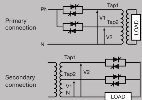
The operating region of control will determine the number of taps required but a maximum of 4 is usually sufficient.
