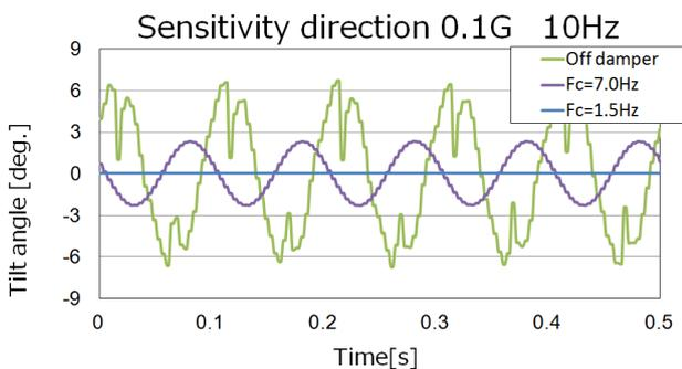
ESC3000Z series implements the digital filter that would remove external noise to give the user a choice of certain filter factor from 16 available settings. Existing inclinometers have to be add extra electrical low-pass filter or mechanical damping structure. ESC30xxZ apply digital filter. It makes wider choice of cut-off frequency and easy to design frequency response. Note: Frequency response is set before shipping. Programmable function will be option.
