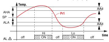
The maximum and minimum temperature alarms can be disabled by setting the related parameters RHR and  $\textit{RLR} = \mathbf{oF}$ . The temperature alarms are signalled lighting up the alarm LED ( $\triangle$ ) and, if configured, also with the buzzer
