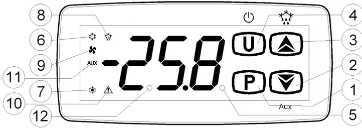
**1 - Key P** : Used for setting the Set point (press and release) and for programming the function parameters (hold pressed for 5 sec.) In programming mode is used to enter in parameters edit mode and confirm the values. In programming mode it can be used together with the UP key to change the programming level of the parameters.
