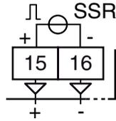
**Logic level 0:**  $V_{out} < 0.5 \text{ VDC}$
