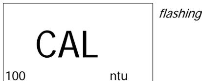
Then the LCD display will return to normal measurement screen, now the meter is finished the calibration procedures ( 0 NTU, 100 NTU calibration ) completely and ready for the measurement.
