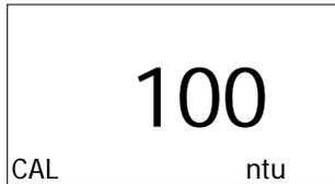
The meter is ready for " 100 NTU " calibration.
