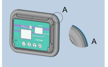
3) Rinse with water at a maximum temperature of 100 °C: direct a low pressure jet toward the components, at an angle of approximately 45° and a distance of at least 300 mm to avoid damaging the seals; pay particular attention to the points indicated in the figure.
