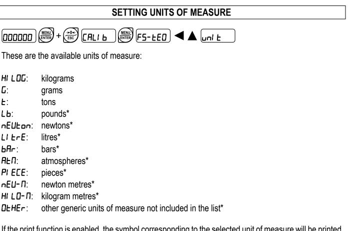
If the print function is enabled, the symbol corresponding to the selected unit of measure will be printed after the measured value.
