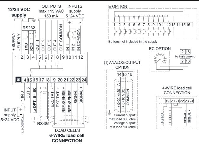
5 outputs: controlled by setpoint values or by remote device via protocol.
