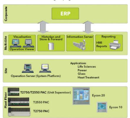
Information Manager provides system connectivity between the control network and the enterprise making data accessible to the entire organization. Enterprise clients systems can be distributed across multiple geographical and organizational boundaries, while maintaining access to any process value via the Operations Server or Information Manager. This allows applications to be
