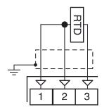
Input circuit: Current injection (150 µA).
