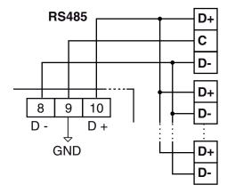
Interface type: Isolated (50 V) RS-485; Voltage levels: According to EIA standard;
