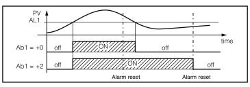
3. An "Acknowledgeable" alarm is an alarm that can be reset even if the conditions that generated the alarm are still present. Alarm acknowledge can be done only by an external command ( button, digital inputs or serial link).
