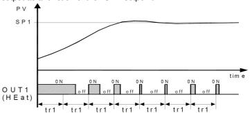
To obtain a good stability of the variable in fast processes, the "tr1" cycle time must have a low value with a very frequent intervention of the adjustment output.
