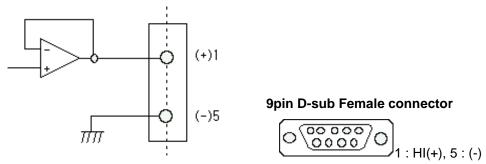
%This Voltage output is proportioned on weight calibration and outputs 0~10V.
