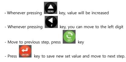
Step 4. Measure/Adjustment optimal Zero balance of Scale
