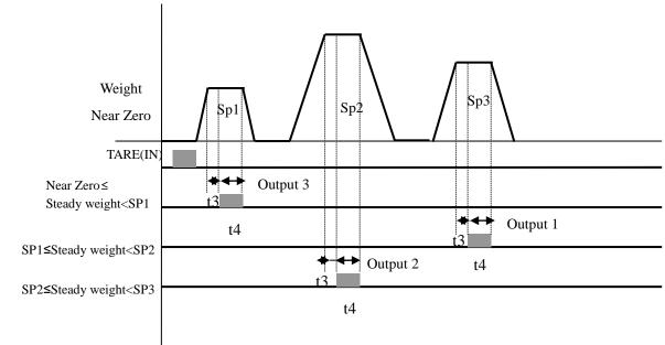
♦ Weighing Mode 3. Checker Mode 1 – Simple Comparison
