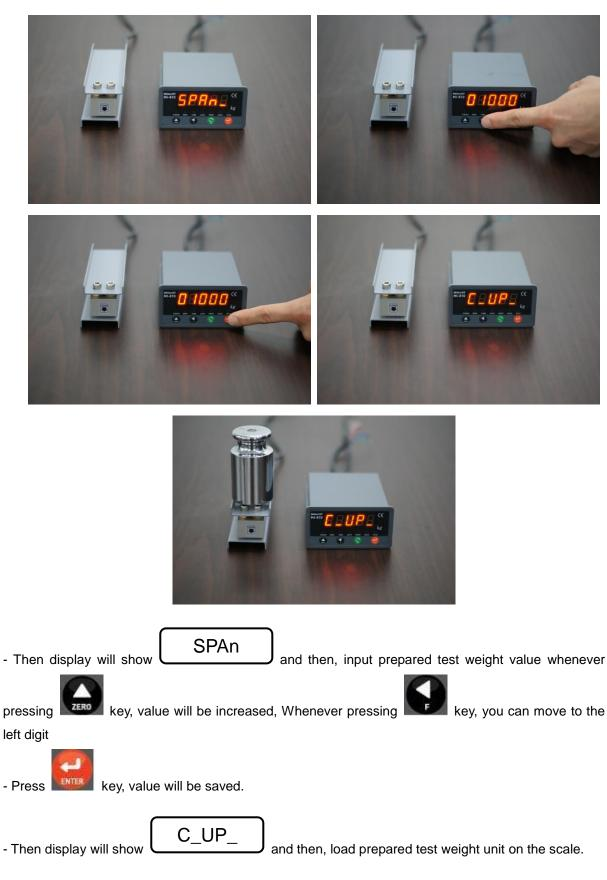
Step 5. Input Prepared Test weight value and load on the Scale.
