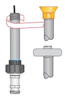
Mount the conduit base onto the adapter and secure the assembly with the locking ring.
