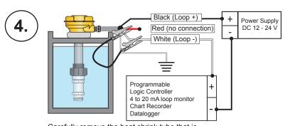
Carefully remove the heat shrink tube that is protecting the red wire. Short the RED and WHITE wires together for 15 seconds. mA should go to 3 to 6 mA
