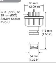
2250 Hydrostatic Level Sensor
