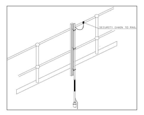
This mounting system has galvanised parts and is designed to be a budget option for transducer mounting.
