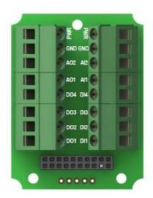
The Power can be connected to either of the PWR and GND terminals.
