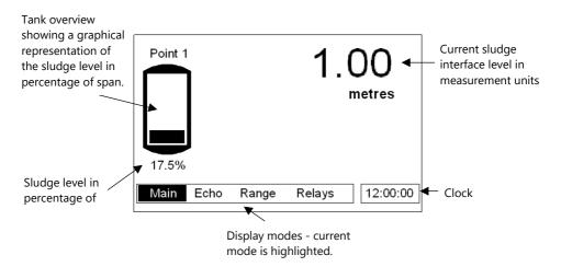
Error messages, such as "Wiper Fault", "Status = LOE" or "Status = Failed" will be displayed on this screen, relating to the point of measure currently being viewed, when a fault condition occurs.
