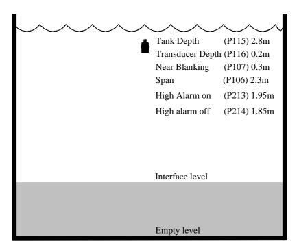
In this example, when the sludge interface level rises to 1.95 m, relay 1 will come on until the level drops to 1.85 m when it will turn off.
