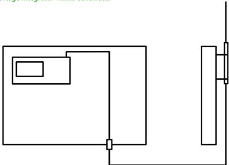
The Integrator on the Bridge should be protected from the elements inside an enclosure, the Antenna extension cable should be installed through a cable gland in the base of the enclosure and out to a suitable position so that the Antenna is above the enclosure.
