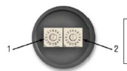
The left dial represents the units of the device. The right dial represents the tens of the device.
