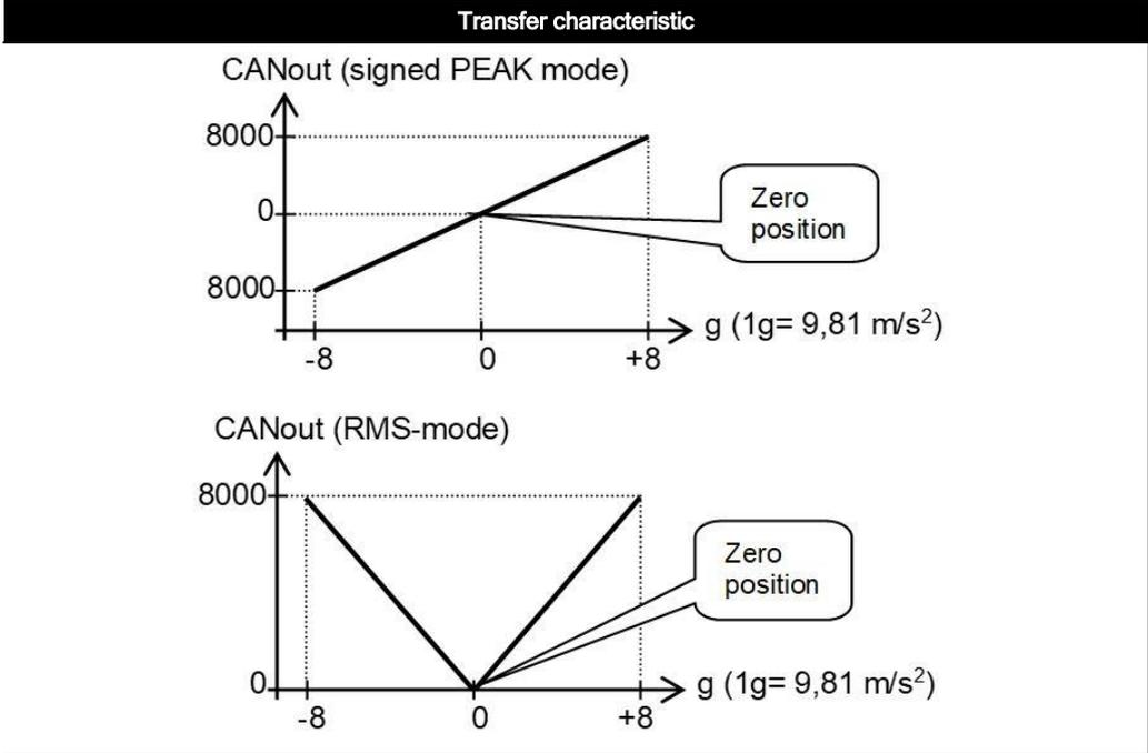
The default 0 g position is when the sensor is mounted horizontal or vertical and no acceleration is applied. The axis parallel to earth gravity will indicate 1 g, the two horizontal axes will indicate 0 g. The two horizontal axes can be zero-ed within  $\pm 5^\circ$  tilt (by the CAN object dictionary) to eliminate mounting offsets. The axis parallel to earth gravity cannot be zero-ed. Optional the axis parallel to earth gravity can be compensated for 1 g gravity by the CAN object dictionary
