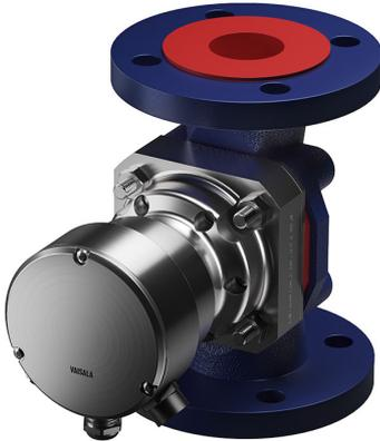
The Vaisala Polaris PR53W valve-body process refractometer is designed to measure concentrations of aggressive chemicals, such as sulfuric acid, hydrochloric acid (HCl), sodium hydroxide (NaOH), and hydrofluoric acid (HF) in production pipelines such as in the chemical, biochemical, and pharmaceutical industries. The PR53W is mounted in a membrane-lined valve body that has no metallic wetted parts. This allows convenient flange mounting to 1 and 2 inch ANSI and DN50 and DN25 flanges.
