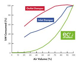
From the data, it can be clearly seen that using methods such as dampers to restrict the airflow is much less efficient than controlling the speed of the fan using an Optidrive Eco HVAC.
