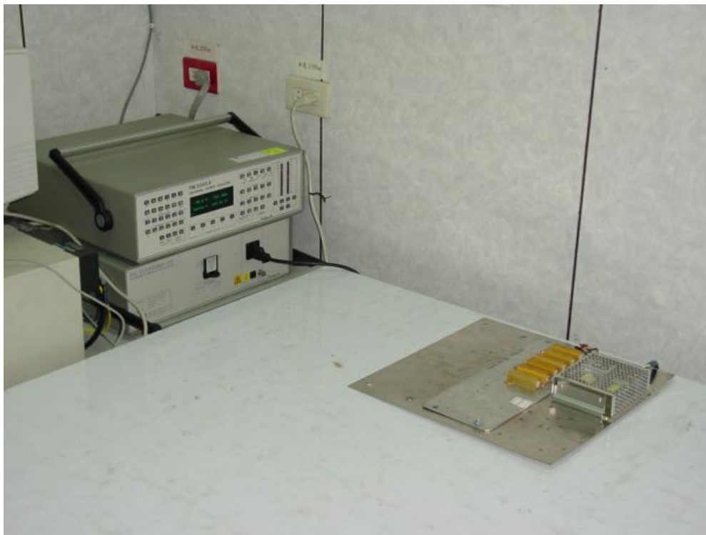
Figure 4.5: Equipment set-up for harmonic testing
