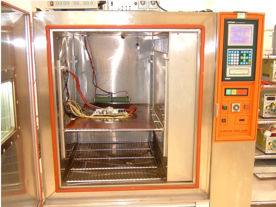
Figure 6.4 Picture of ambient tester (chamber)
