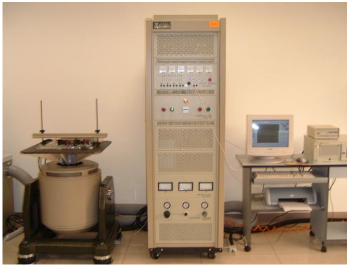
Figure 2.10: Instruments for vibration test
