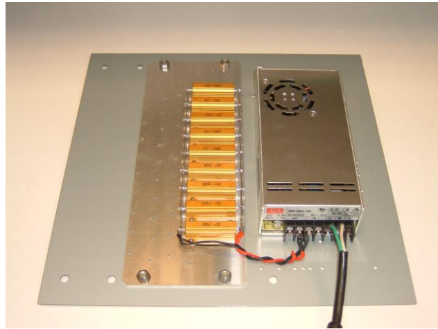
Figure 5.1: Standard setup for EMC test
