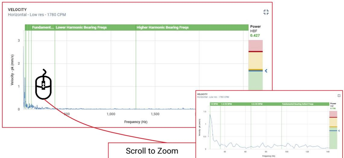
When a band is in an alarm state, the whole band will change colour to indicate where the issue is. If you hover over the band, the *power level* on the right-hand side will show the magnitude of the vibration for that band, and how far into the warning level the value is.
